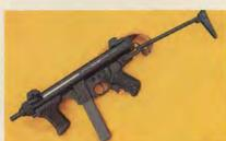
ABOVE: Field-stripped Beretta Model 12S. Disassembly can be done in matter of seconds by removing barrel butt and end cap. LEFT: Beretta Model 12S with stock extended. First produced in 1959, Domenico Salza's design is compact, lightweight and accurate.
